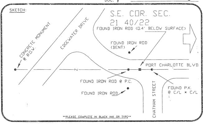
REFER: P.B. 6, PG. 21A&B BASIS OF BEARING-PLAT DATA REFER: F.B. 279-12 All bearings and distances must be from the corner to the witness. Indicate whether corner was found, set, or replaced and show north arrow.
