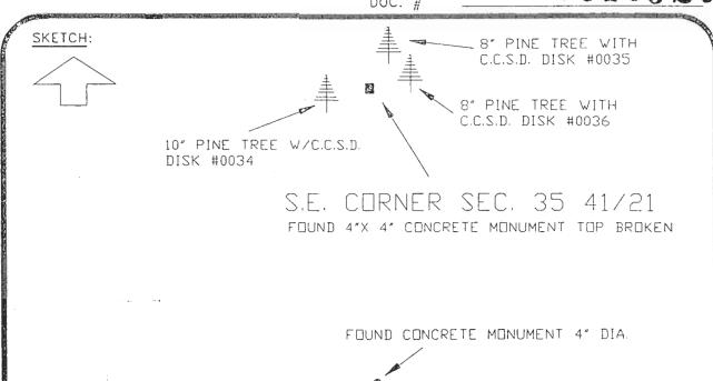
ROTONDA SPRINGS SUBD., PLAT BOOK 12, PG. 5 REFER: F.B. 274-29 All bearings and distances must be from the corner to the witness. Indicate whether corner was found, set, or replaced and show north arrow. BASIS OF BEARING-SOLAR OBSERVATION SET SURVEY MARKER POST 2.0' N.'LY REFERENCE MEASUREMENTS ( at least three vicinity references must be given below even if they appear on the above sketch ):
