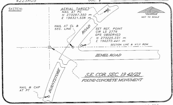
REFER FB 292/75 BASIS OF BEARING SOLAR OBSERVATION All bearings and distances must be from the corner to the witness. Indicate whether corner was found, set, or replaced and show north arrow.
