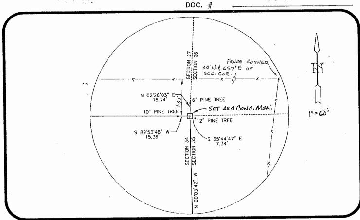
All bearings and distances must be from the corner to the witness. Indicate whether corner was found, set, or replaced and show north arrow.
